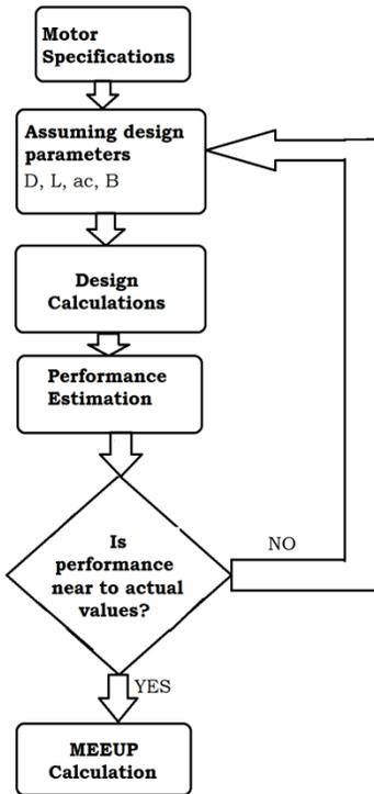
Fig. 1. Calculation procedure to find out real generator parameters
