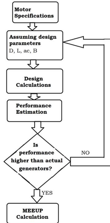
Fig. 2 Calculation procedure for proposed generator
