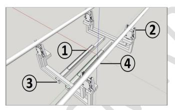
Fig.2: 2. Telescopic Slider, 2.Gripper Module, 3.Support Chassis, 4.HV Line
