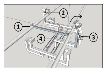
Fig.2: 1. Spacer, 2.U-Grooved Wheel, 3.Gear Assembly, 4.Main Chassis [8]
