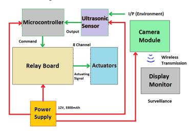
Fig.3: Block diagram of Electronic Circuitry
