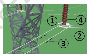
Fig.1: 1. Tower, 2.Bundled Conductors, 3.Suspension Clamps, 4.Vertical String Insulators [8]
