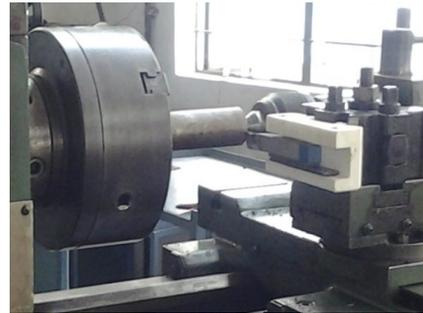
Fig. 10: Experimental set up for turning with RPT tool holder
