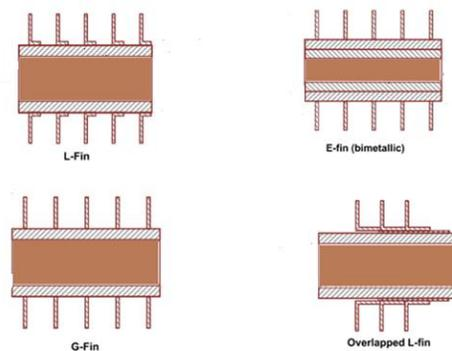
Fig. 2 Different types of Fins [1]
