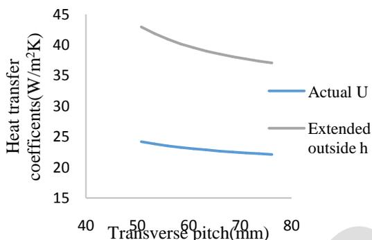
Fig. 4 The graph of different heat transfer coefficient vs transverse pitch
