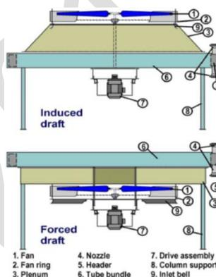
Fig. 1 Basic configuration of induced & forced type air cooled heat exchanger
