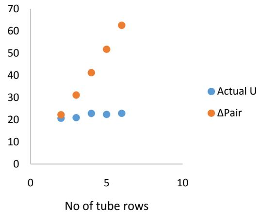
Fig. 7 The graph of actual U and Pressure drop vs no. of tube rows
