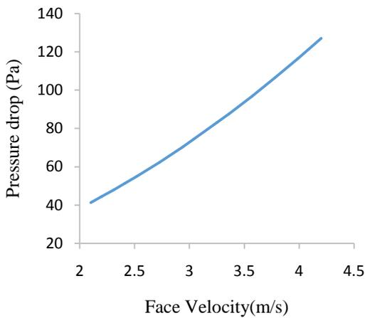
Fig. 5 The graph of pressure drop vs face velocity
