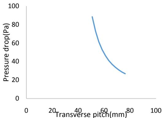
Fig. 3 The Graph of pressure drop vs transverse pitch
