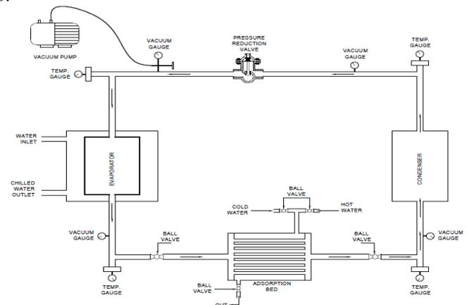
Fig. 2 Schematic diagram of experimental setup of solar assisted adsorption water chiller
