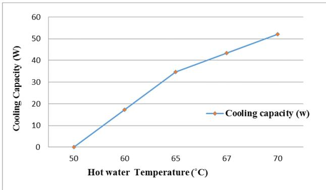
Fig. 4 Hot Water Temperature Influence on Cooling Capacity (W)
