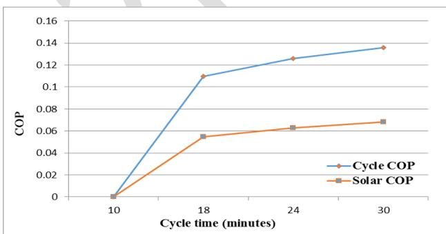
Fig. 7 Cycle time influence on cycle COP and solar COP
