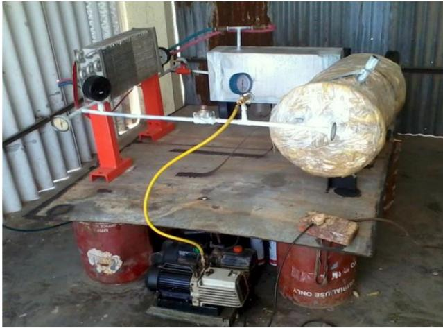
Fig. 3 Experimental setup of solar assisted adsorption water chiller
