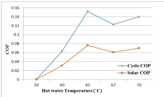
Fig. 5 Hot water temperature influence on cycle COP and solar COP
