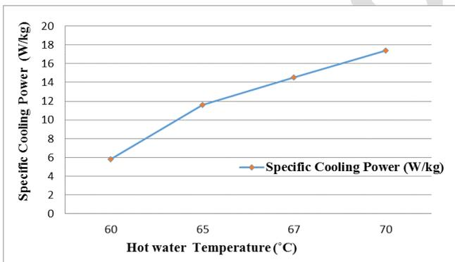
Fig. 6 Hot water temperature influence on specific cooling power
