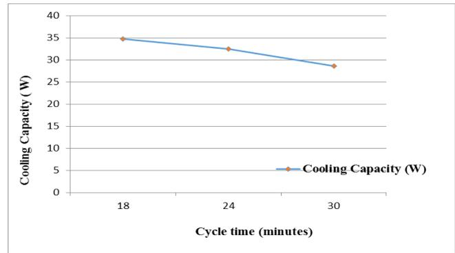
Fig. 8 Cycle time influence on cooling capacity (W)
