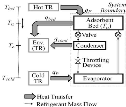
Fig. 1 Schematic diagram for an ideal simple adsorption cycle. [4]
