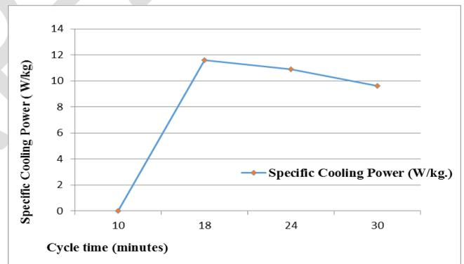
Fig. 9 Cycle time influence on specific cooling power (SCP)
