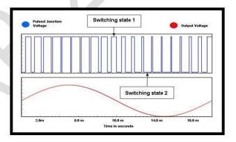
Fig. 12 Unipolar (Two Level) Switching Scheme
