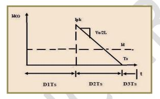
Fig. 8 Diode D<sub>4</sub> Current
