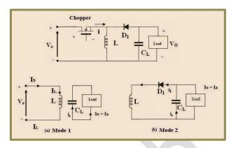
Fig. 3 Circuit diagrams of Buck Boost converter, Mode 1 and Mode 2
