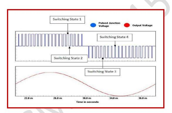
Fig. 14 Unipolar (Four Level) Switching Scheme
