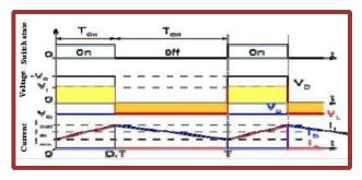
Fig. 4 Current and voltage waveforms in continuous mode
