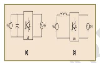
Fig. 10 Voltage source inverter (a), Current source inverter (b)
