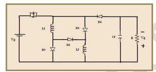
Fig. 6 Switched Inductor Buck Boost Converter
