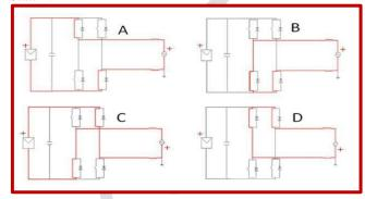
Fig. 15 A-Current Path for Full Bridge Converter implementing Unipolar Switching Scheme
