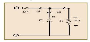
Fig. 9 Current flows through Diode D 4
