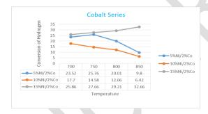
Fig 2 shows the effect of temperature on hydrogen conversion for cobalt series
