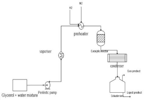
Fig.1. Schematic of glycerol steam reforming setup
