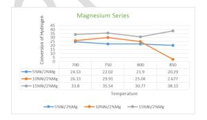
Fig 3 shows the effect of temperature on hydrogen conversion for magnesium
