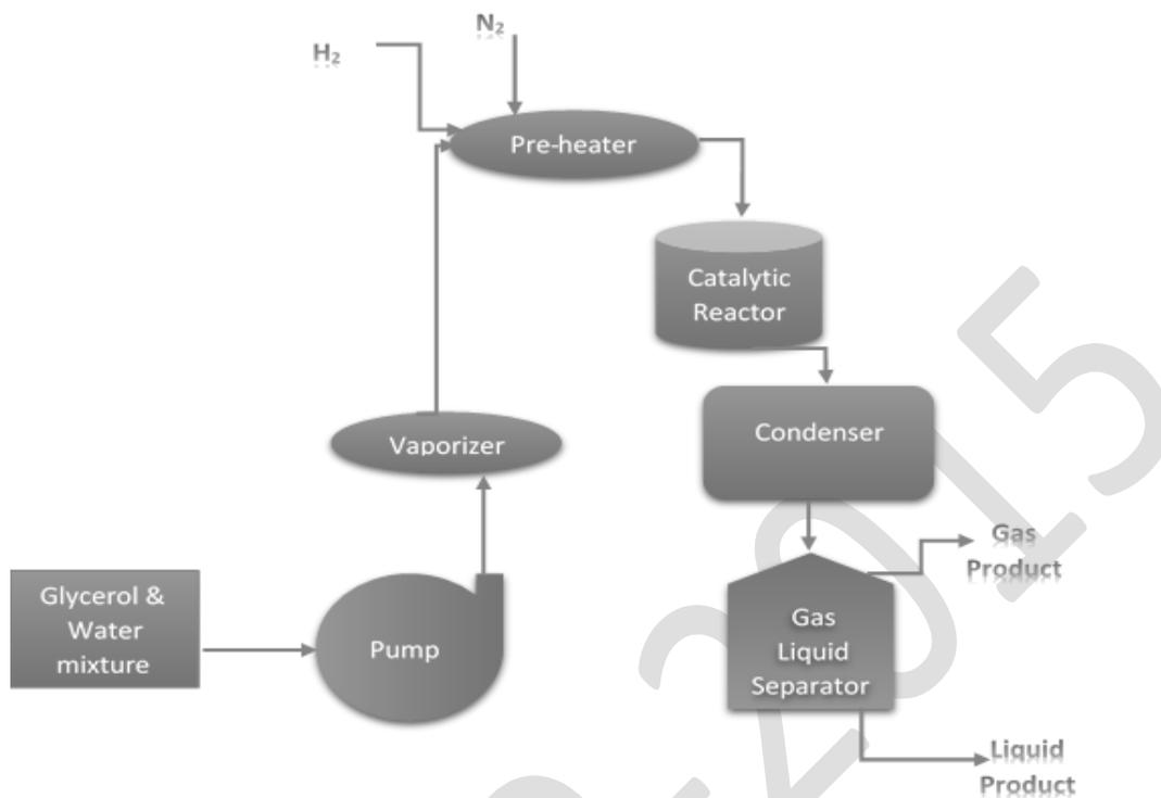
Fig.1. Schematic of glycerol steam reforming setup
