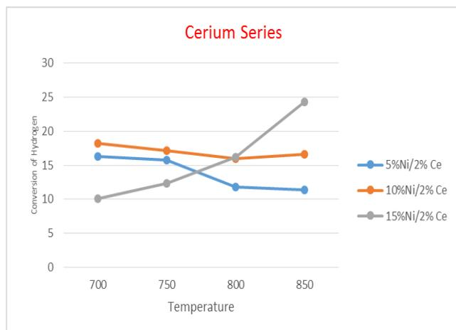
Fig 3 shows the effect of temperature on hydrogen yield for cerium series.
