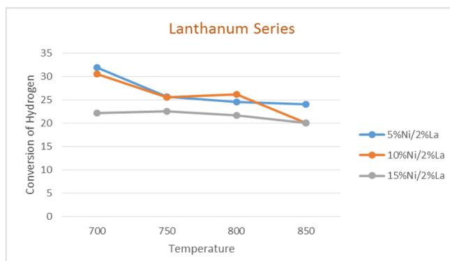
Fig 2 shows the effect of temperature on hydrogen yield for lanthanum series.
