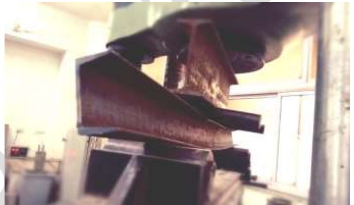
Fig. 5 Buckling of Channel section 'without Lip'
