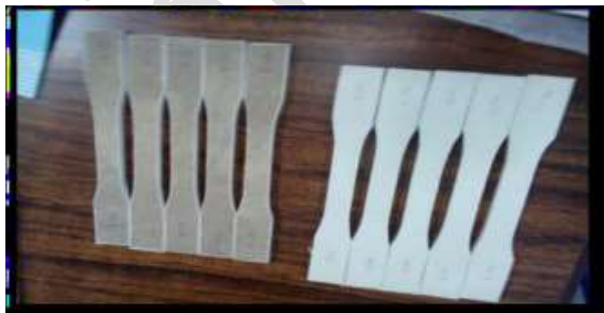
Fig: 5 Test sample of hybrid and jute laminate
