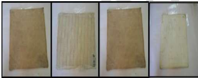
Fig 1: Laminates (i) jute with 9 layers, (ii) hybrid with 13 layers of bamboo and glass (iii) Jute with 17 layers (iv) Glass with 28 layers
