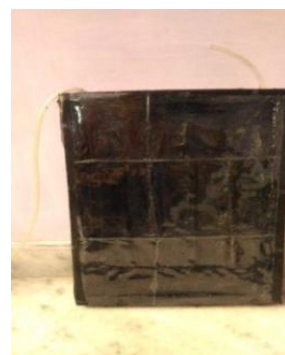
Fig. 2.2 Stainless steel FPC with Glazing
