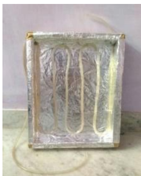
Fig. 2.1 Aluminium FPC with Polymer tube
