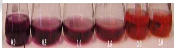
Fig.1 Reaction of fluoride in the range 0.0–3.0 mg L -1 with 2 \times 10^{-4} M of fluoride reagent.
