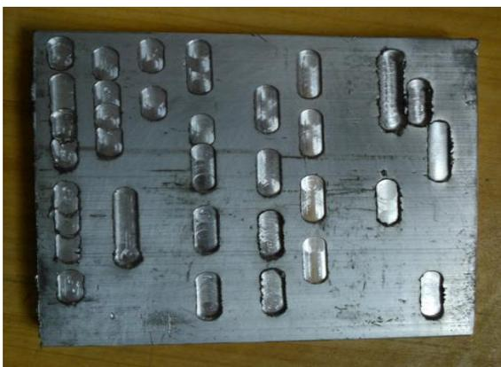
Fig. 1.5: Work-piece after 27 experiments
