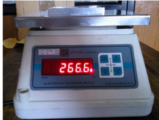
Fig. 1.6: Digital weighing m/c indicating Reduced weight of the work-piece
