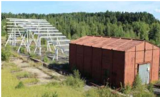
Fig. 4. Stationary HEMP simulator ALLUR of High-Voltage Scientific-Research Center of Federal State Unitary Enterprise Russian National Electric Technical Institute (Istra, Moscow Region). Overall dimensions: 100m x 35m x 13.5m; displacement volume: 10m x 10m x 10m; pulse shape: 2.5/25 nanoseconds; maximum strength of electric field pulse: 70 kV/m.
