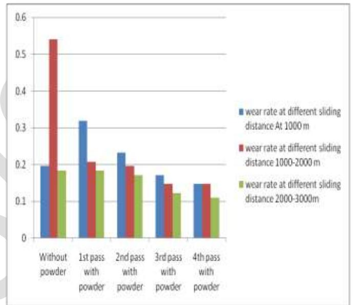
Fig 3. Wear rate graph at different sliding distance
