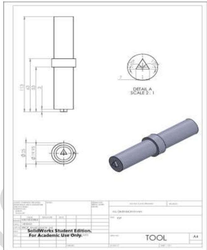
Fig. 2. Tool Drawing at Solid Works.
