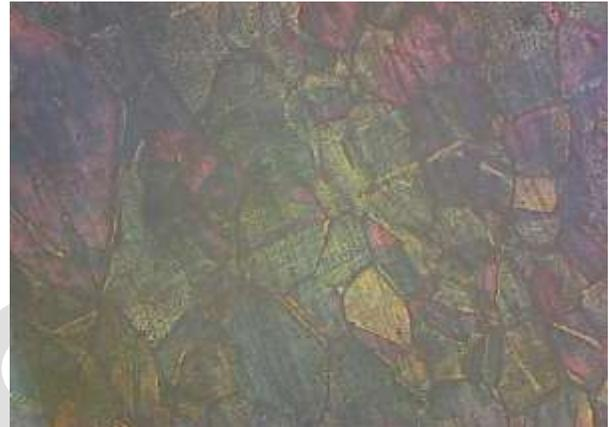
Fig 6. Base Metal without processing at 100X
