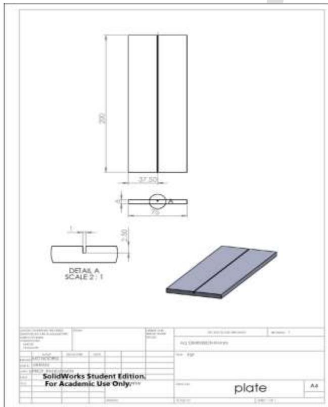
Fig. 1. Copper Plate Drawing at Solid Work
