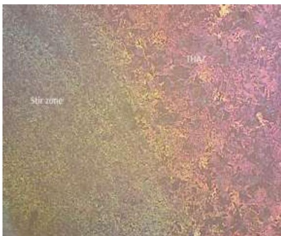
Fig 8. Specimen with GP single passes at 100X
