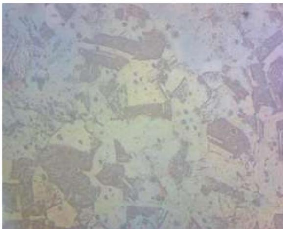
Fig 7. Specimen without GP with single pass at 500X
