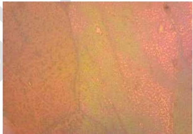
Fig 6. Base Metal without processing at 500X
