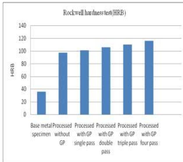
Fig. 3. Rockwell hardness number (HRB) Vs No of passes
