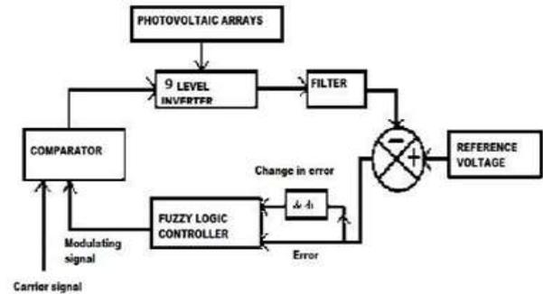
Fig.5 Block Diagram of Inverter and Fuzzy logic
