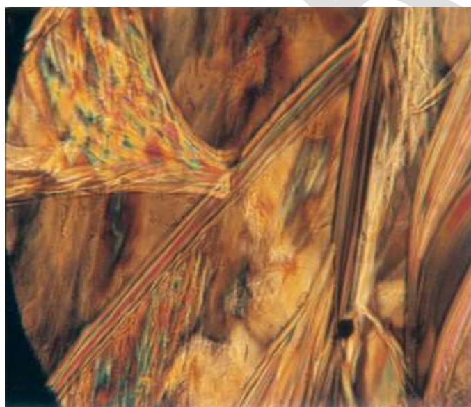
Fig.1. "POM Texture", on cooling the mesophase of compound 5b.
