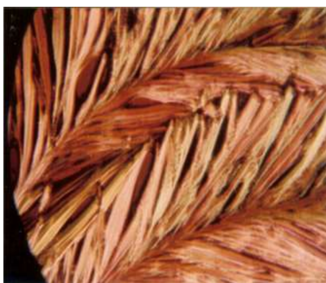
Fig.2. "POM Texture", on cooling the mesophase of compound 5e.
