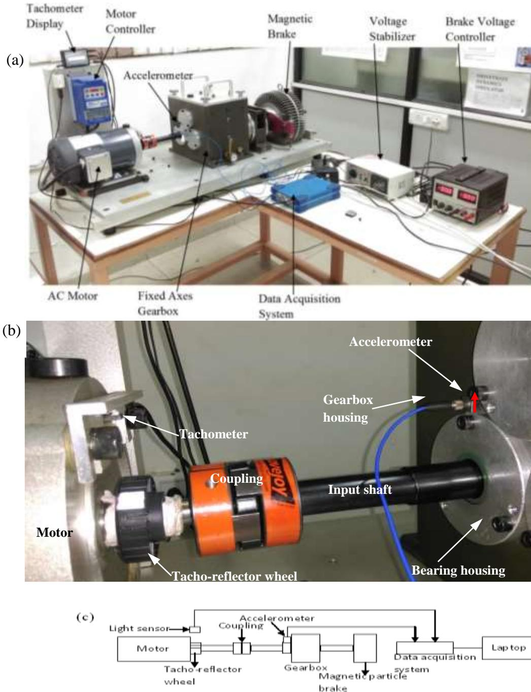
Fig. 3. (a) Drive train diagnostic simulator (b) sensor arrangement and (c) functional diagram
