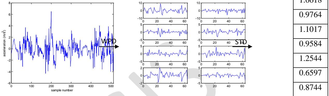
Fig. 6. A data sample from the synchronized vibration signal for the healthy pinion, the 8 frequency bands and standard deviation values of wavelet packet coefficients
