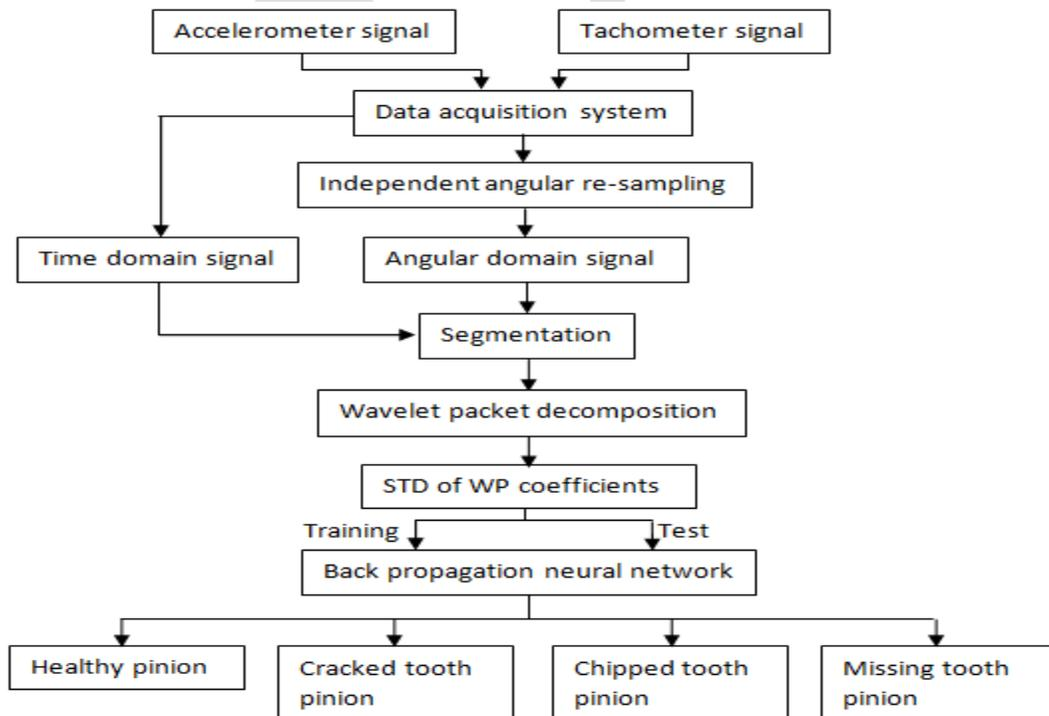
Fig. 1. Flowchart of the proposed fault diagnosis procedure
