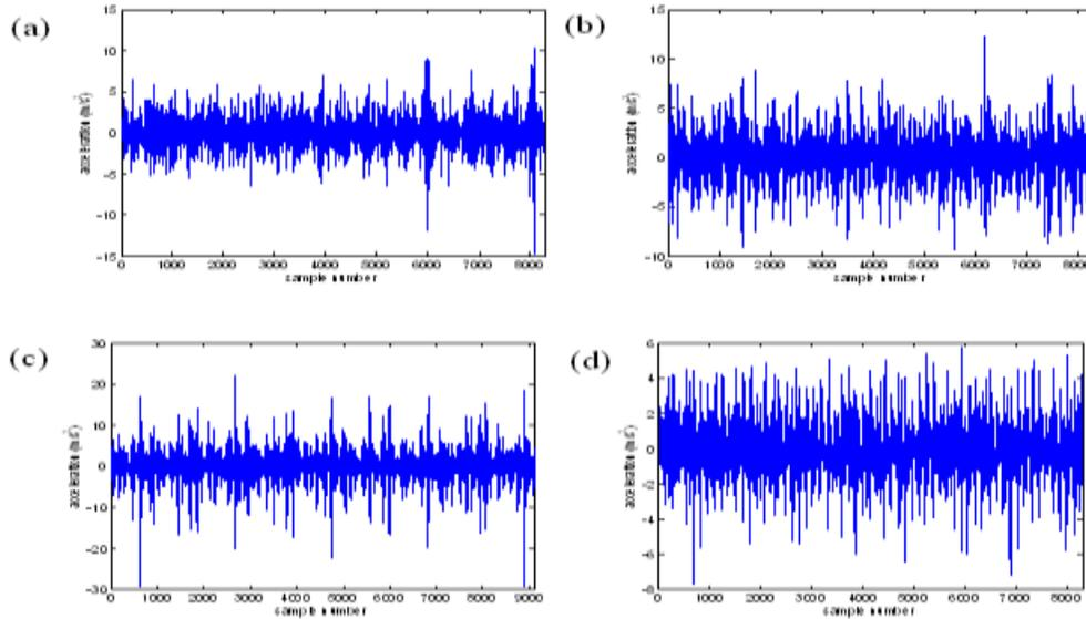
Fig. 4. Vibration signal acquired from the gearbox with (a) healthy pinion, (b) cracked tooth pinion, (c) chipped tooth pinion and (d) missing tooth pinion
