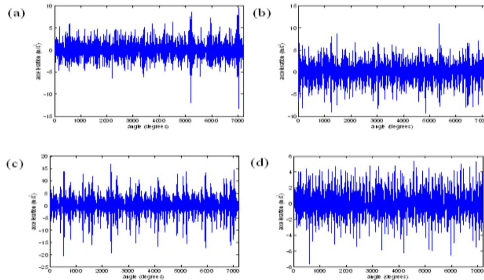
Fig. 5. Synchronized angular domain vibration signal for the gearbox with (a) healthy pinion, (b) cracked tooth pinion, (c) chipped tooth pinion and (d) missing tooth pinion
