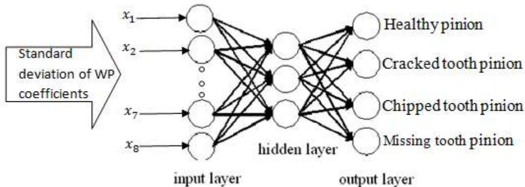
Fig. 7. Concept of multi-layer perceptron model
