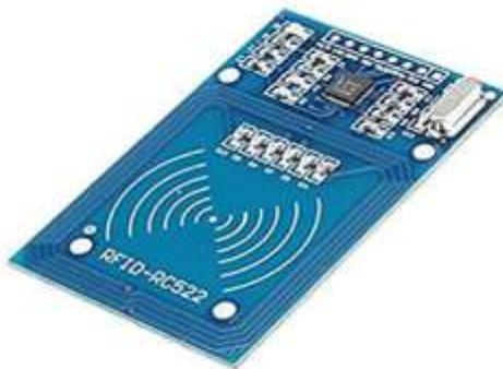
Product Specification MF RC522 is applied to the 13.56 MHz non-contact card chip.
