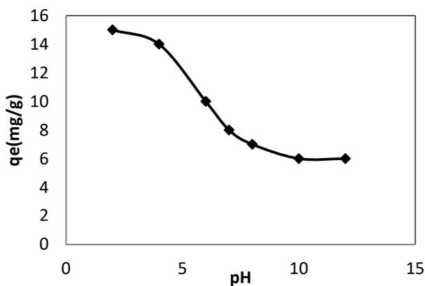
Fig. 7 Effect of pH on adsorption at 20 ppm concentration of BBR
