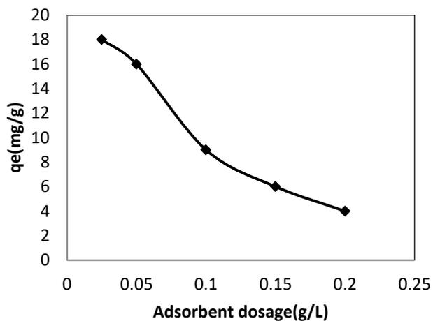
Fig. 5 Effect of adsorbent dosage on adsorption of BBR
