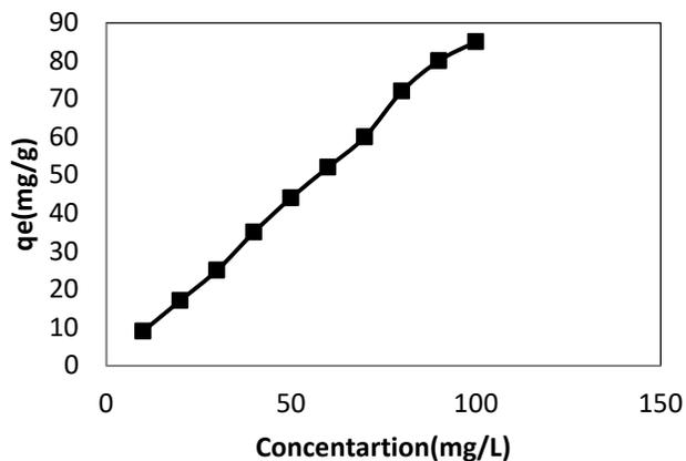
Fig. 4 Effect of initial dye concentration on adsorption of BBR
