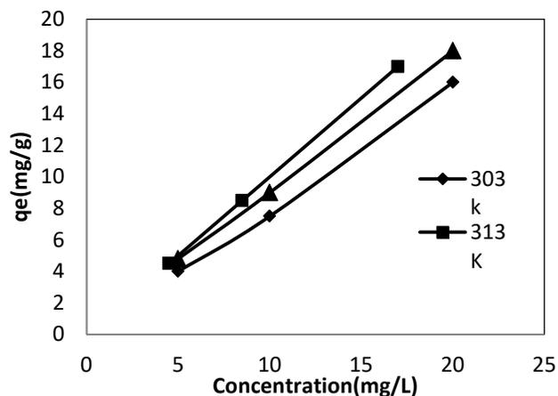
Fig. 6 Effect of Temperature on adsorption of BBR
