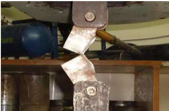
Fig. 12 (c): crack propagation reaches to full rupture. [12]
