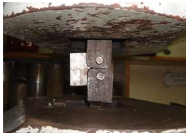
Fig. 11: C(T) specimen loaded on UTM for fracture testing. [12]
