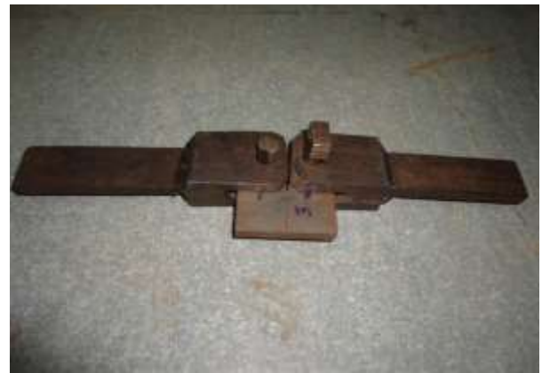
Fig 10: C(T) specimen with pin and fixtures. [12]
