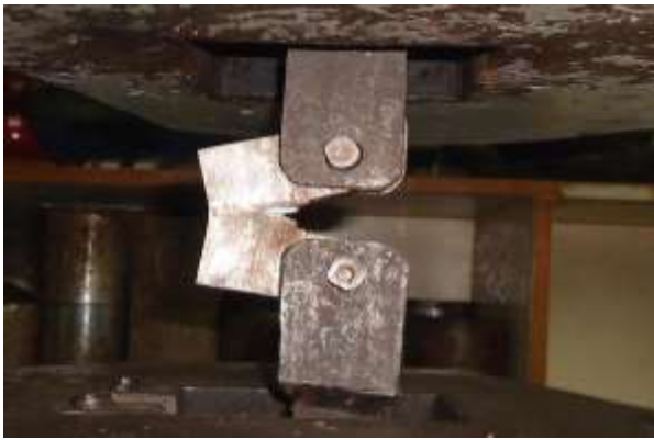
Fig. 12 (a): crack propagation commenced. [12]
