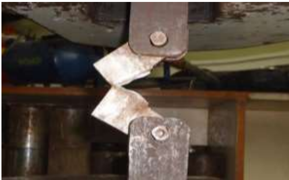
Fig. 12 (b): crack propagation advances. [12]
