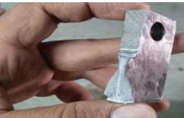
Fig. 13: C(T) specimen piece after full rupture. [12]
