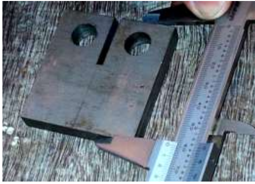
Fig. 8: Compact Tension (C(T)) specimen made of SA-516 (before testing)
