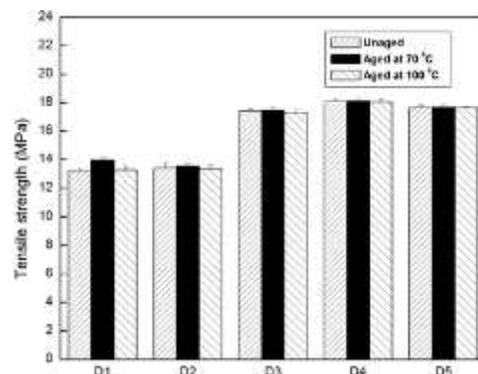
Fig. 5 Variation in tensile strength before and after ageing of the NR vulcanizates containing DCBS
