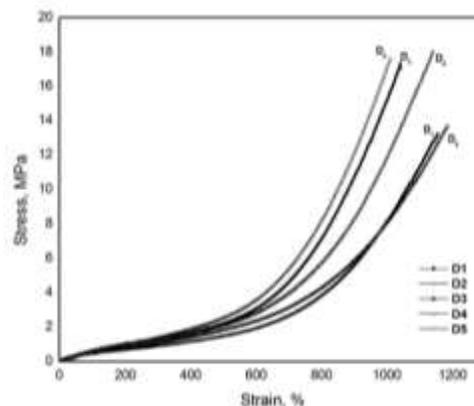
Fig. 3 Stress-strain curves of the NR vulcanizates containing DCBS
