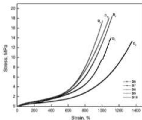
Fig. 4 Stress-strain curves of the NR vulcanizates containing DBBS
