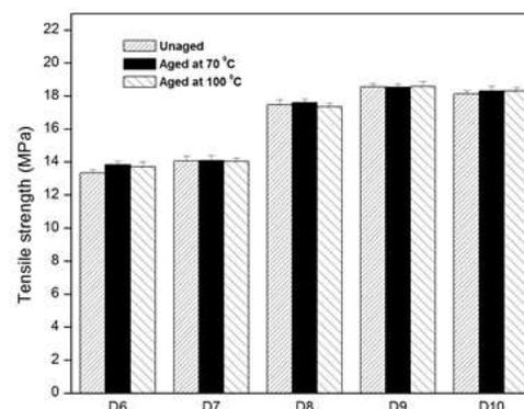
Fig. 6 Variation in tensile strength before and after ageing of the NR vulcanizates containing DBBS
