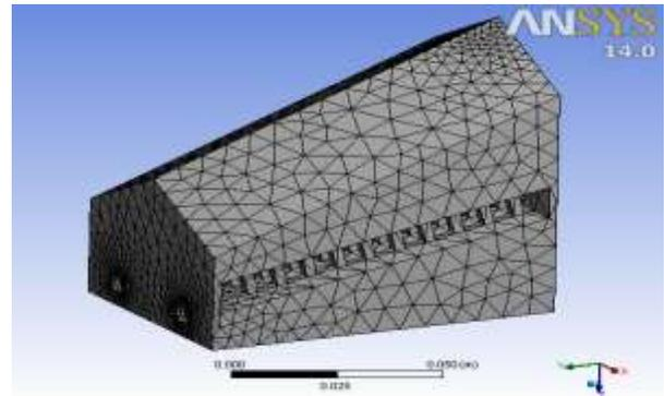
Figure 3. Mesh domain of the solar dryer.
