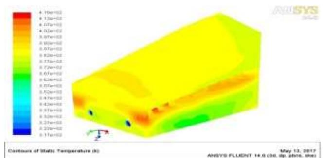
Figure 13. Temperature variations on solar green house dryer at 2:00 pm
