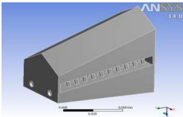
Figure 2. 3D Model of Modified Green House Solar Dryer.
