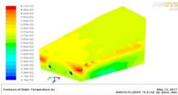
Figure 14. Temperature variations on solar green house dryer at 4:00 pm
