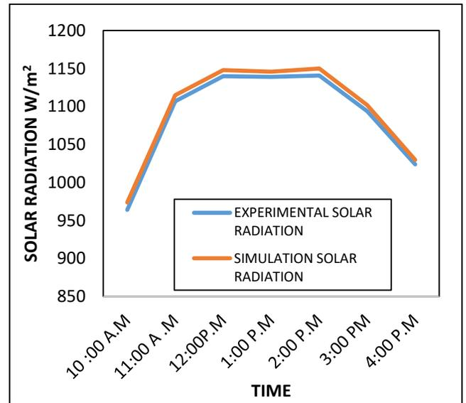
Figure 5. Results of solar radiation for the solar green house dryer in time
