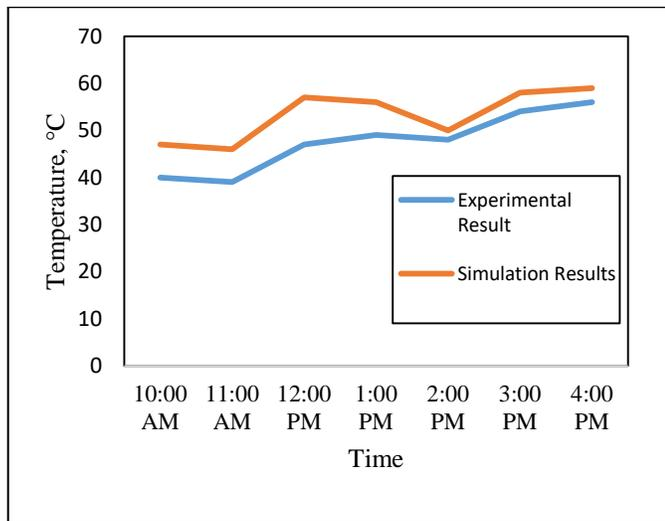
Figure 4. Results of variation in temperature for the solar green house dryer with variation in time
