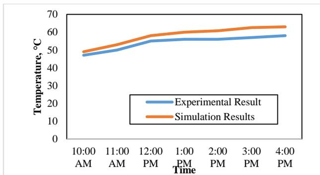
Figure 10. Result of temperature for the natural convection solar dryer with time (natural convection)
