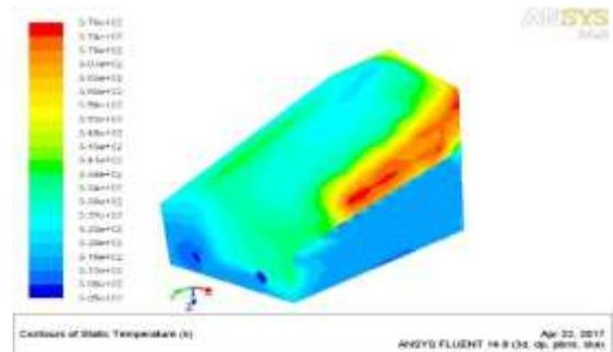
Figure 6. Temperature variations in solar green house dryer at 10 am under forced convection
