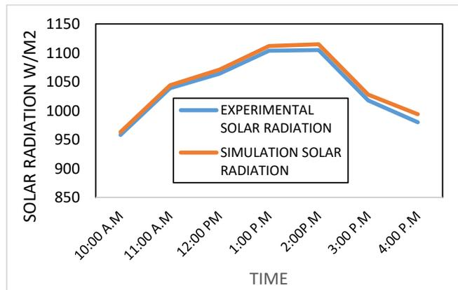
Figure 15. Variation of solar radiation with time (natural convection)
