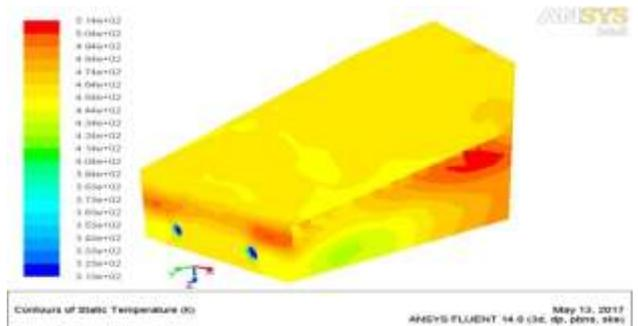
Figure 11. Temperature variations on solar green house dryer at 10 am
