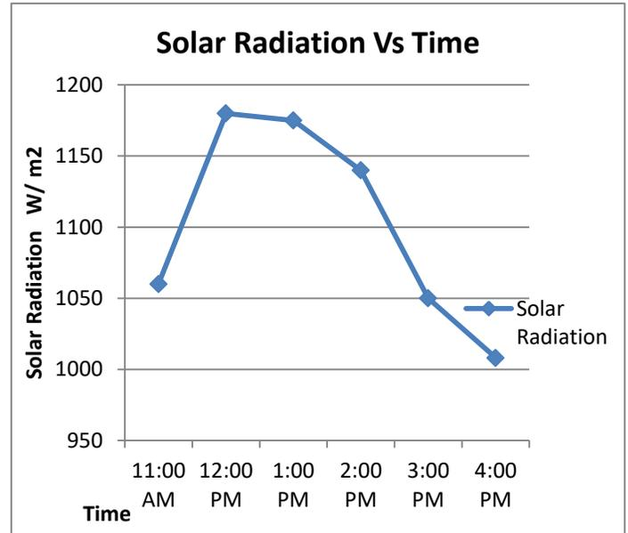
Fig. 3: variation in solar radiation with time
