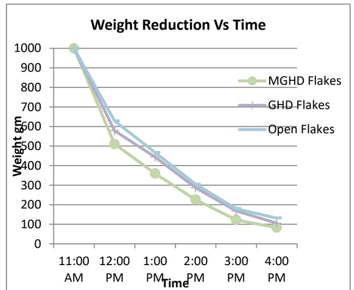
Fig. 7: Drying curve for different mode of drying
