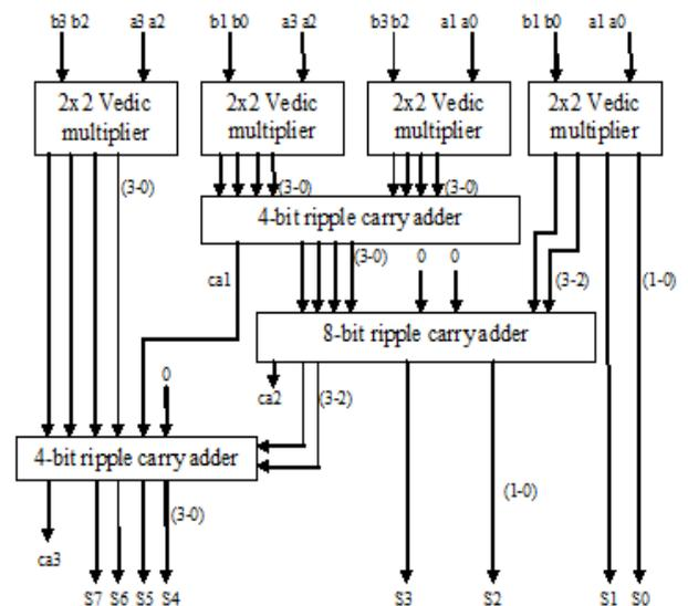
Figure 5: Block diagram of 4x4 Vedic multiplier
