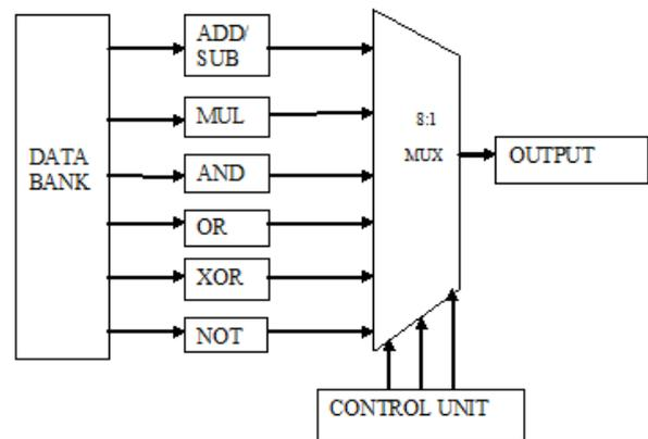
Figure 1: Block diagram of proposed Arithmetic Logical Unit
