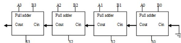
Figure 2: Block diagram of Ripple Carry Adder
