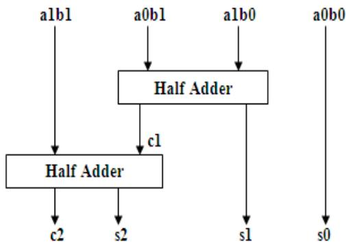
Figure 4: Block diagram of 2x2 Vedic multiplier
