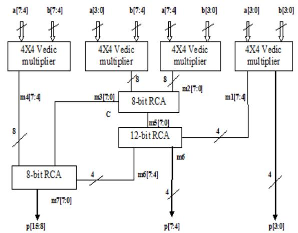
Figure 6: Block diagram of 8x8 Vedic multiplier
