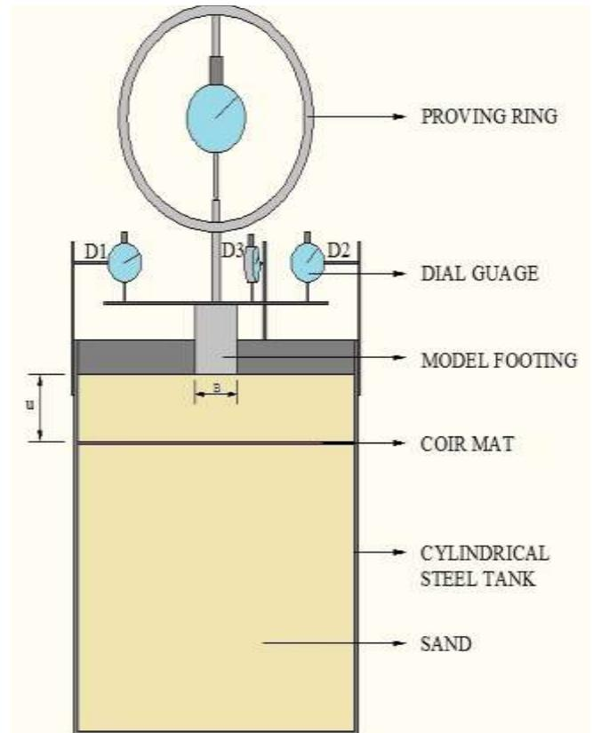
Fig.1: Typical layout of Reinforced sand
