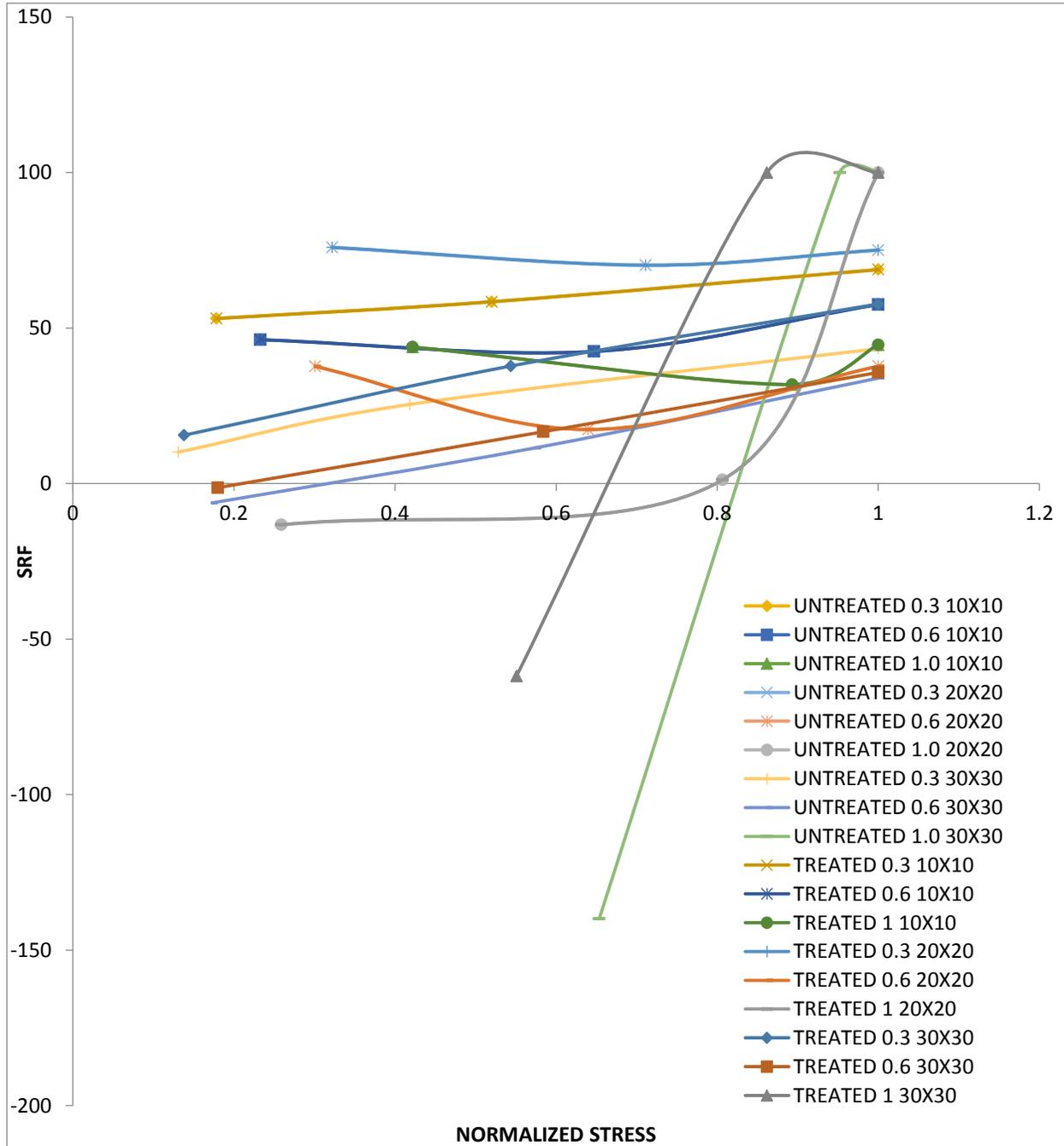
Fig 2: SRF vs Normalized settlement for untreated and surface treated coir mats at different u/B ratios.
