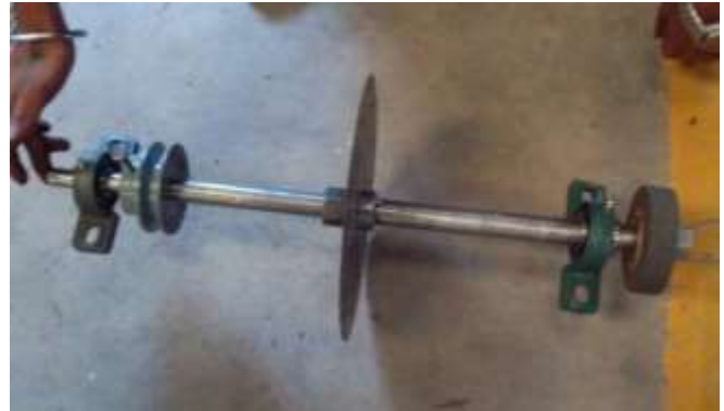
Fig. 11 Circular Shaft (Small Shaft)
