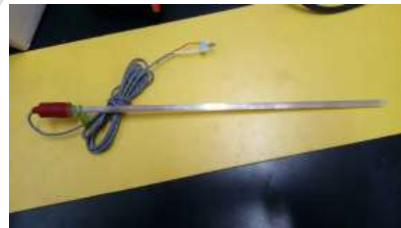
Fig. 7 PT-100 Temperature sensor
