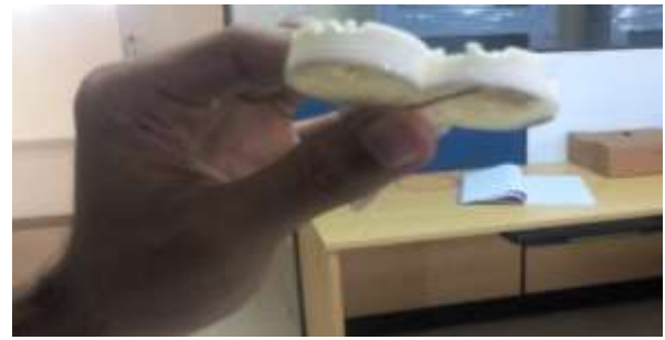
Fig. 10 Part before vapor smoothing treatment
