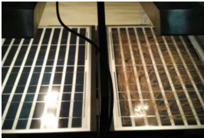
Fig. 3 Shows laboratory set up for clean panel and dusty panel
