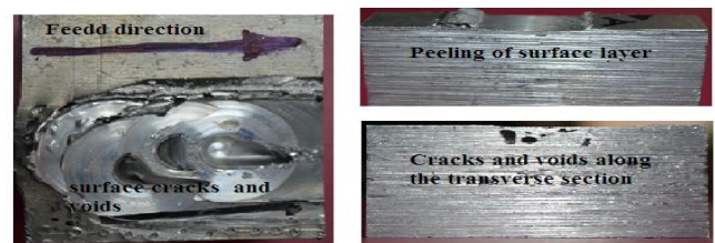
Fig.4 shows the macrograph the friction stir processed failed SMMC during higher feed rates above 60mm/min.
