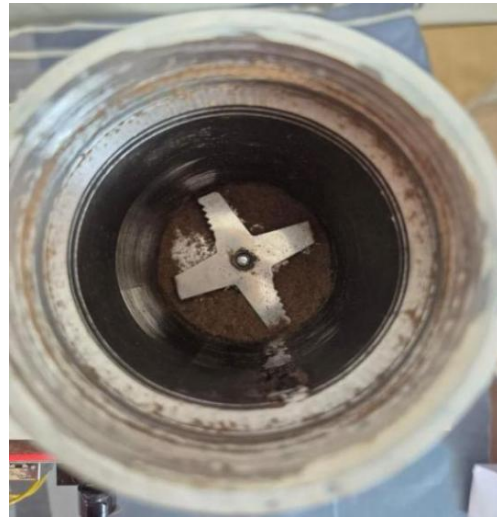
Figure 4.2 Grinding chamber with blade
