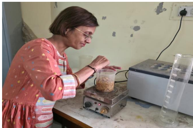
Picture 3: Chemical Activation Process with Phosphoric Acid
