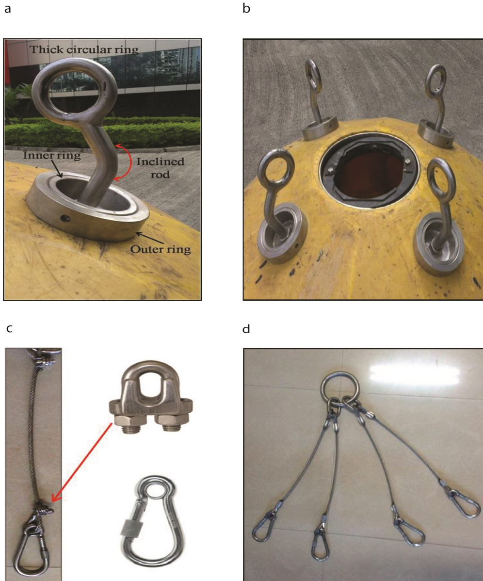
Figure 5: Design and reinforcement of components for lifting and deployment of the dome: a) SS Hook-loop assembly. b) Hook-loop assemblies. c) SS Wire rope & Snap-hook. d) SS Wire rope & Snap-hook set.
