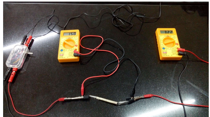
Fig.6a: Test circuit using Portable power supply
