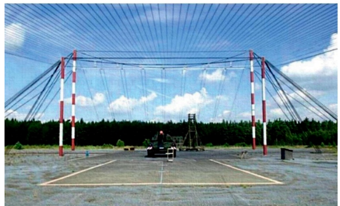
Fig. 2. Typical design of a guided-wave test bench to simulate HEMP impact (in particular, E1 component of HEMP).
