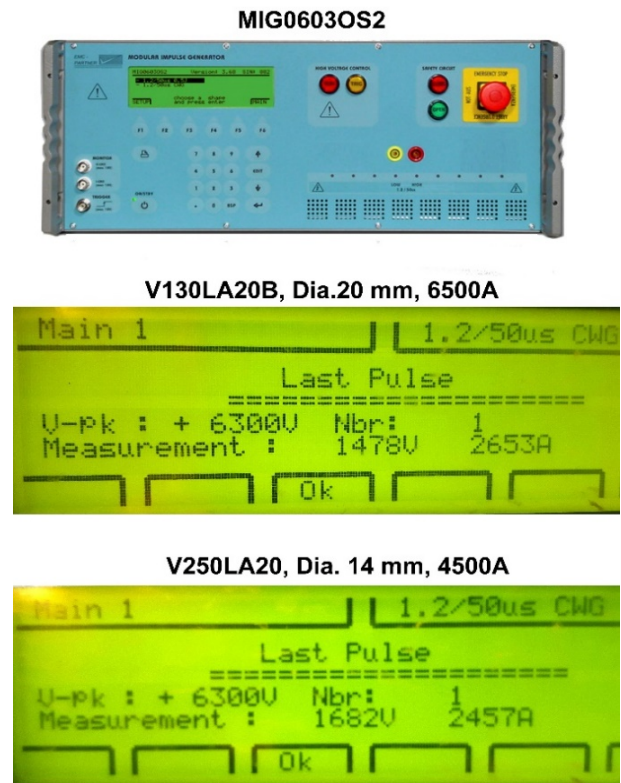
Fig. 3. Screenshots of MIG0603OS2 pulse generator when testing varistors V250LA20 (14 mm) and V130LA20B (20 mm) with maximum rated pulse current at 4,500 A and 6,500 A, respectively.
