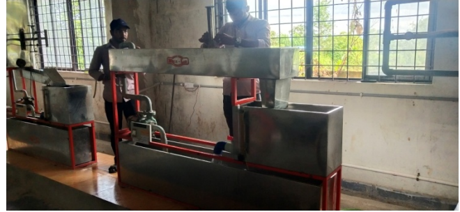
Fig.2. Experimental View of Trapezoidal Notch.
