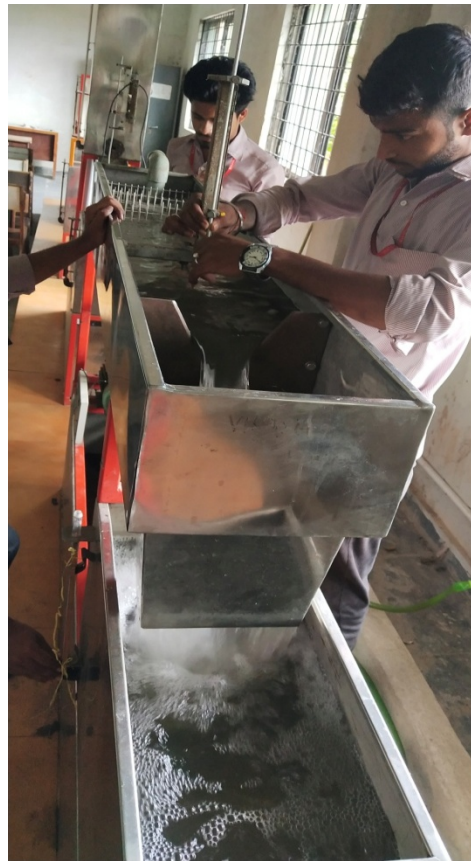
Fig. 2. Experimental view of notch apparatus
