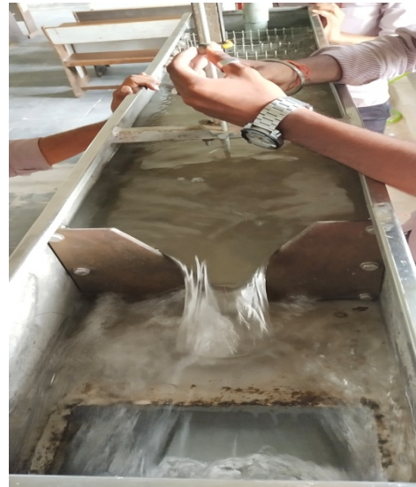
Fig. 1. Experimental view of V-notch section
