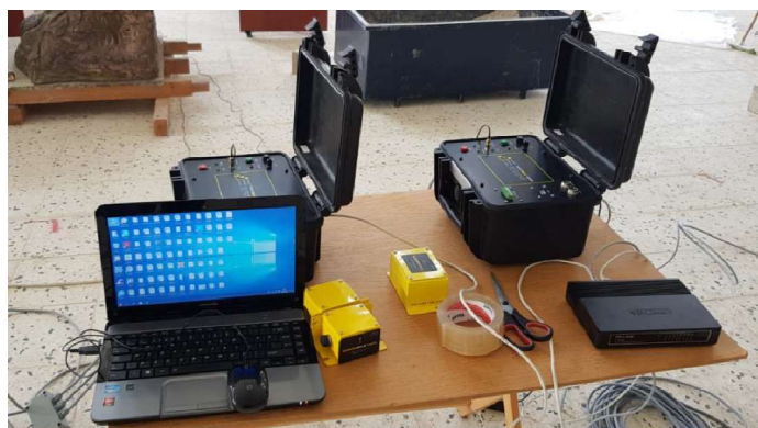
Fig 5. Datalogger and accelerometers
