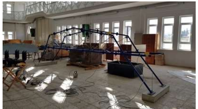
Fig 3. Model steel bridge
