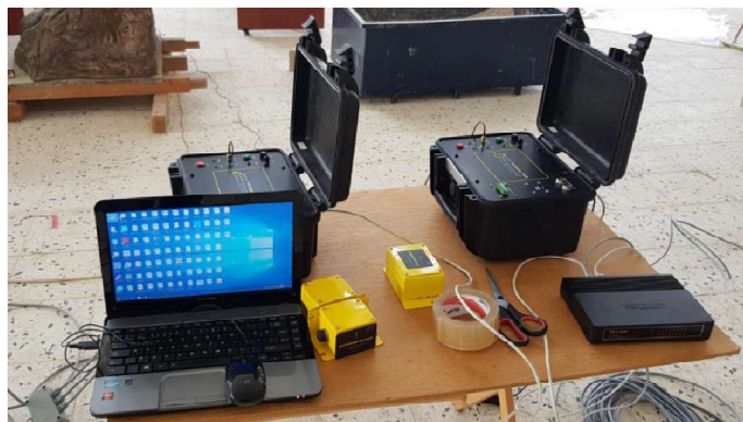
Fig 4. Datalogger and accelerometers
