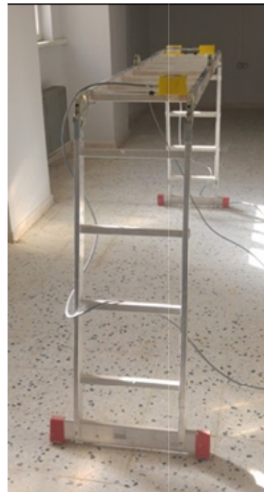
Fig. 4. Measurement of aluminum benchmark bridge with accelerometers
