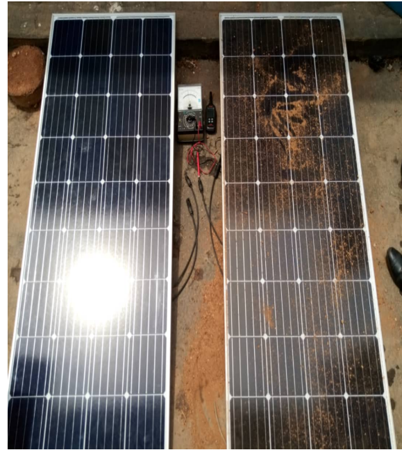
Figure 1: Clean and dusty photovoltaic modules.
