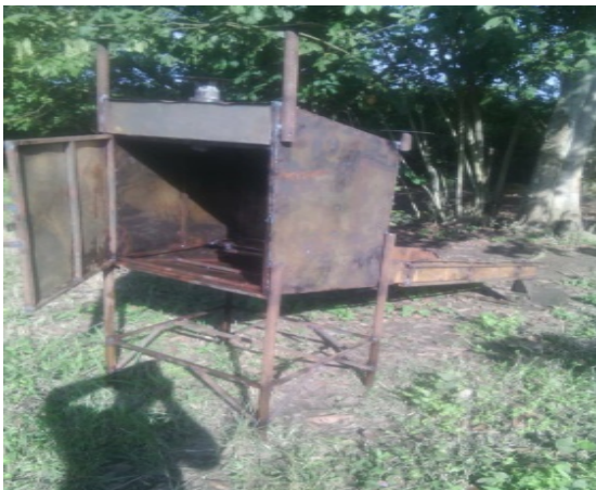
Figure 1: Side view of hybrid solar dryer under construction
