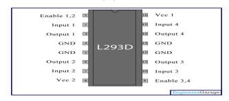
Motor drivers act as an interface between the motors and thus the control circuits. Motor require high amount of current whereas the controller circuit works on low current signals. Therefore the function of motor drivers is to need a low current control signal then turn it into a higher-current signal which can drive a motor.
