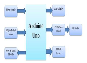
Arduino Uno is based on ATmega 328P microcontroller. It consists of 20 pins out of which 14 are digital pins and the rest 6 are PWM. It can be programmed using a computer on Arduino IDE. Arduino being open sourced, has a really good community which makes development very convenient and any kind of problems are taken care of by the community. We are using it because it is
