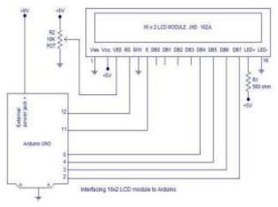
The digital input lines (DB4-DB7) are interfaced with the Arduino pins from 5-2. To adjust the contrast of the display here we are using a 10K potentiometer. The current through the back LED light is from the 560-ohm resistor.
