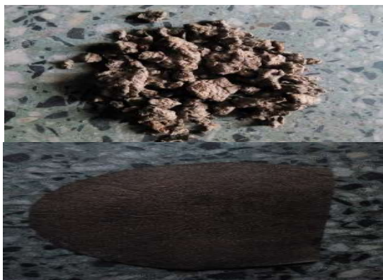
Figure 5: Showing unbleached EFB Pulp Samples and Pulp Sheets from MEA Process
