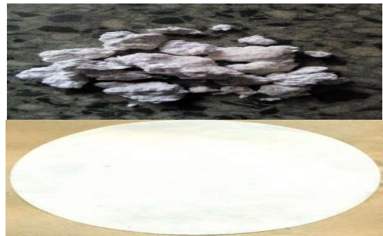
Figure 6: Showing EFB Pulp Samples from MEA Process Bleached to 16.2 Kappa Number and Pulp sheets
