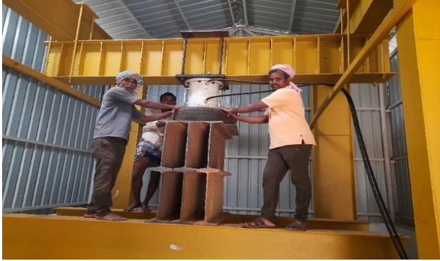
Fig 22 Keeping the tyre with compacted gravel in loading frame.
