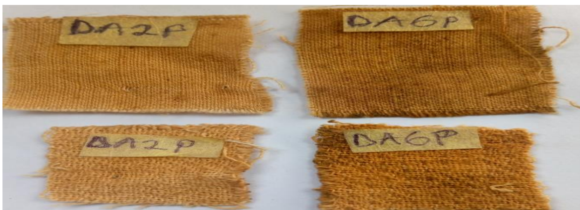
Fig 7: Cotton and wool fabrics dyed with dye extract and tested for perspiration fastness
