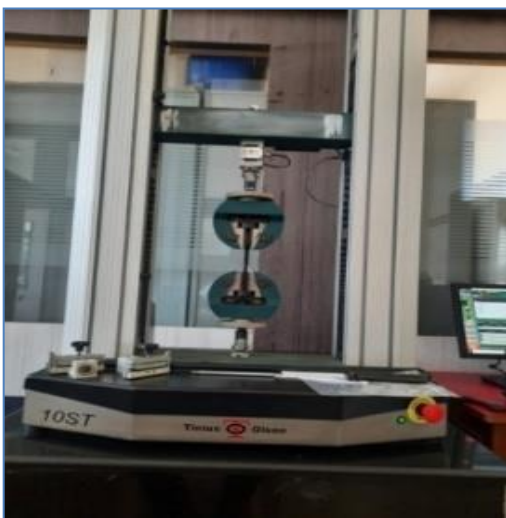
Fig. 6. Tinius Olsn Model 10ST (MUTM).
