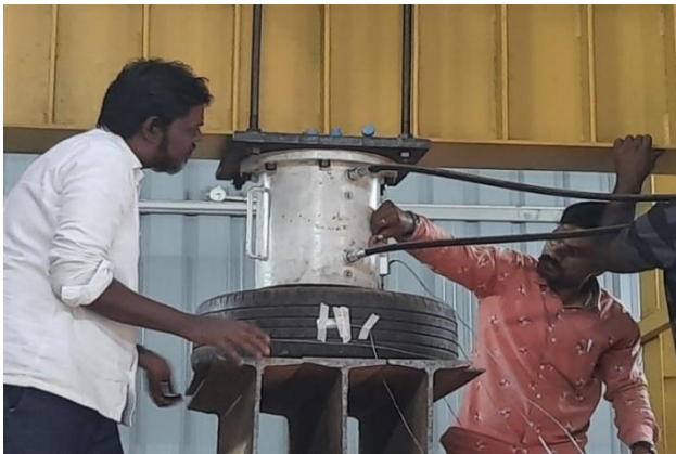
Fig 24 Fixing sensors and LVDT
