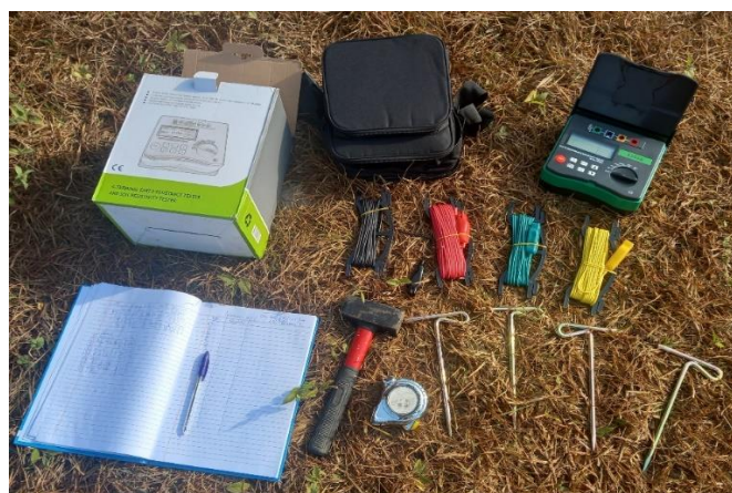
Fig 3 Resistivity Measurement / Test Equipment
